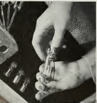
SLIDING A GLASS ENVELOPE WITH EXHAUST TUBE ATTACHED OVER THE ELEMENTS OF A MINIATURE TUBE.
