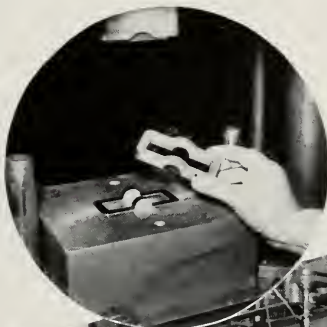
PLASTIC CORE-FRAME FOR A TELEVISION RECEIVER BEING REMOVED FROM HYDRAULIC PRESS.
