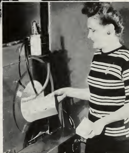
MACHINE SPRAYS MAGNESIUM OVER SMALL PIECES OF MICA USED FOR INSULATORS IN MINIATURE TUBES.
